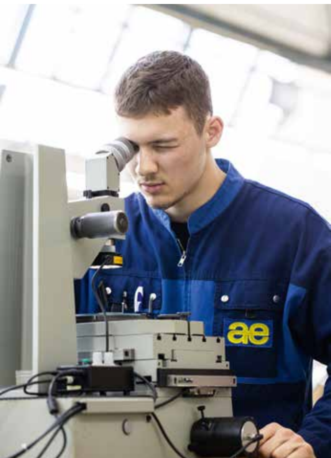
The watch screws are inspected under a microscope using an in-process measuring system.
