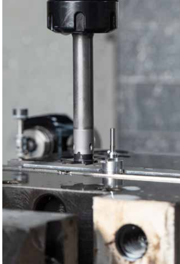
The HORN circular milling system is used for cut-off milling.
