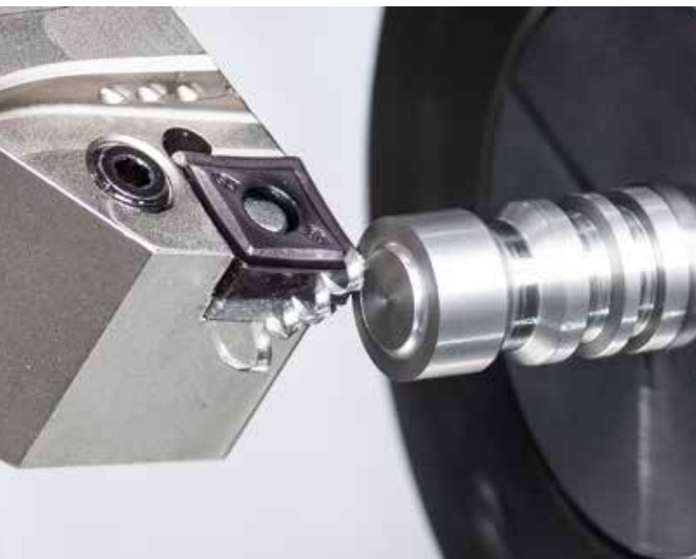
An ISO tooling solution from Boehlerit is used for longitudinal turning of the nozzle.
