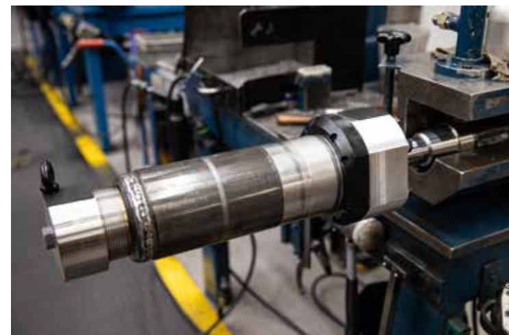
Assembly of the hydraulic cylinder used in the moving floor systems.
